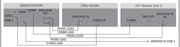
The G68 can copy the currently selected audio and video inputs to two different outputs, called COPY ZONE 2 and ZONE 3, for recording, or for controlling one or two other rooms. For example, a G51 Receiver could be used in a second room to listen to a source connected to the G68.
