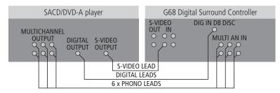
The G68 Digital Surround Controller provides eight analogue inputs, three of which can be used as a multichannel input from a source with a suitable analogue multichannel output, such as an SACD player.
