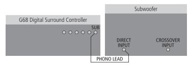
The Meridian SW1600 and SW5500 subwoofers provide both digital and analogue inputs, allowing you to connect them to either the digital or analogue subwoofer outputs of the G68. The analogue connection must be used if you do not have a digital main speaker.
