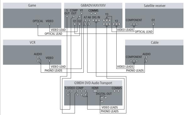
If you are using the G68ADV, AXV, or XXV Digital Surround Controller in conjunction with a G98DH DVD Audio Transport, you can perform video switching in the G68 but take advantage of the video format conversion and scaling in the G98 to drive the display device.
